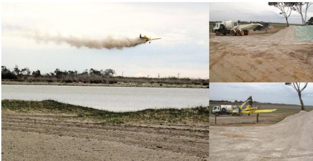
**Figure 26: Left: Aerial application of limestone in Boggy Lake, SA. Right: photos showing mechanism used to upload fine agricultural limestone into the aircraft in a nearby paddock. (From Fitzpatrick et al. 2011d)**
