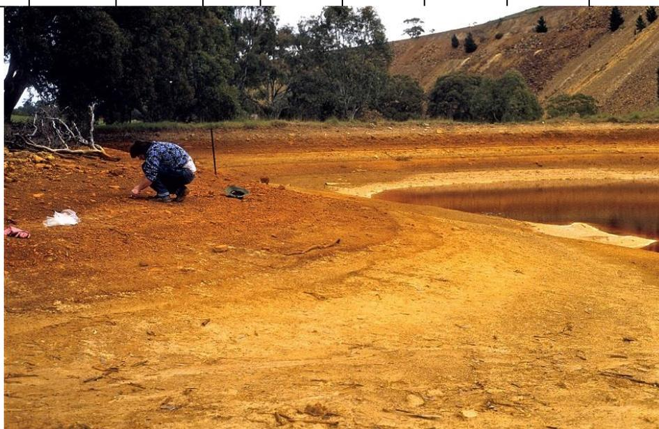
**Figure 113: Photograph of iron-rich precipitates on the sides of the settling pond at the abandoned Brukunga pyrite min (sampled in 1992)**
