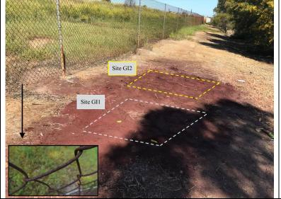
Fig. 2 Photograph of the Anthropogenic acid sulfate soil site on Garden Island. Two field sites (GI1 and GI2) were used for a nine-month fencing trial. The condition of the nearby fence is shown as an inset
