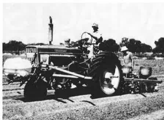
Spray inoculation equipment mounted on a tractor (Photo: R. Gault, CSIRO)
