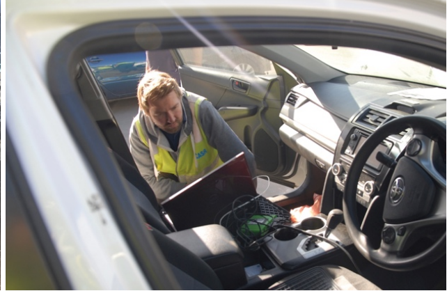
Crashed vehicles at the holding yard (left) and a CASR researcher performing an EDR download via the OBDII port (right)
