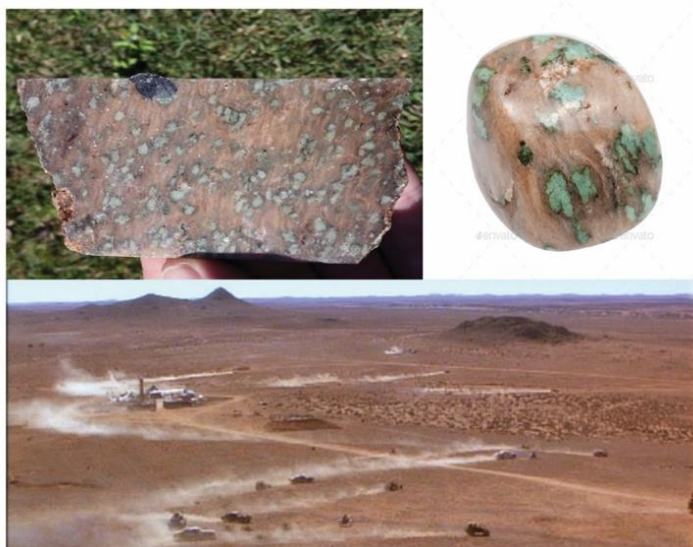
Figure 1. Slab and polished stone of Nundorite. Note the bright green aegirine (sodian pyroxene). Western NSW field area (courtesy of George Miller).
